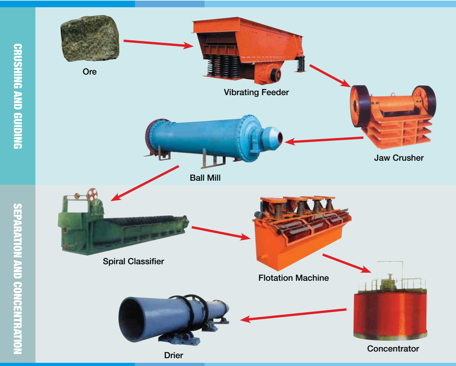
Figure 5. A simplified diagram showing a mineral processing method excluding Smelting and Refining.
